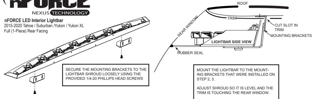
TIGHTEN ALL SCREWS TO SECURE IN PI ACF
