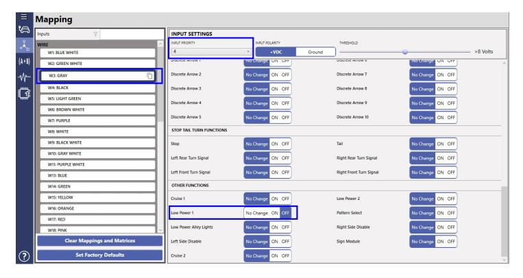
3. From the example in #2, when +V is applied to the gray wire, Low Power 1 will be turned off even if the photo sensor is active since the gray wire control is a higher priority than the photo sensor control.
