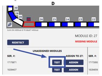
e. Once the module location is verified click Assign to set the ID selected in step C. The application will go through the process of setting the desired module IDs and go through the process of identifying them again.
