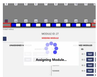
f. Once the module IDs are all identified properly SoundOff Central Lightbar software will show the lightbar without any red missing or unassigned modules.
