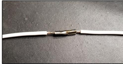
Crimped & Soldered Connection
