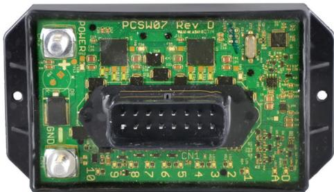
The primary expansion to bluePRINT is the Remote Node. Each remote node adds 10 outputs to the bluePRINT system, as well as 4 inputs that are selectable between a high (positive) or low (ground) signal.
