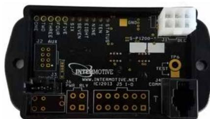
bluePRINT Link utilizes vehicle data harvested from the Controller Area Network Bus, otherwise known as the CAN-BUS.
