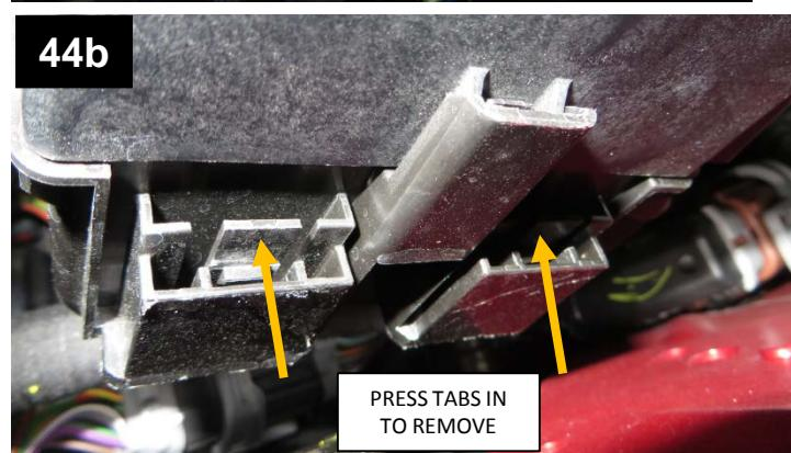
REMOVE BOX ABOVE UPFITTER WIRE LOOM.
