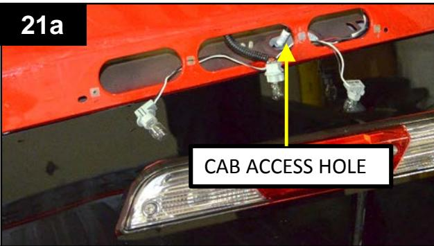
USE 6' OF FISH TAPE TO ROUTE HARNESS – "N" DOWN THROUGH CAB ACCESS HOLE & TOWARD DRIVERSIDE C-PILLAR.
