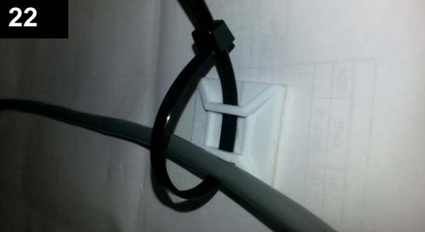
AFTER HARNESS – "N" HAS BEEN PULLED THROUGH HEADLINER, LOOSELY ATTACH (4) ZIP TIES & ANCHORS ABOVE SMALL CONNECTORS. ANCHORS WILL BE USED TO SECURE HARNESS ALONG C-PILLAR
