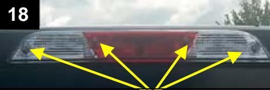
REMOVE "Vehicle CHMSL SCREWS" (4) Torx T-20 or 7 mm socket-HANG ON TO SCREWS. YOU WILL NEED THEM LATER IN THE INSTALLATION IN SECTION NUMBER 28 .
