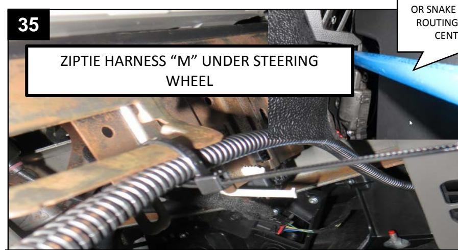
ROUTE POWER & GROUND HARNESS – “M” THROUGH CENTER CONSOLE TO FUSE BOX LOCATED ON PASSENGER SIDE OF VEHICLE. SECURE WIRE HARNESS WITH ZIP TIES. FISH TAPE CAN BE USED AS AN AID TO PULL HARNESS THROUGH CENTER CONSOLE.
