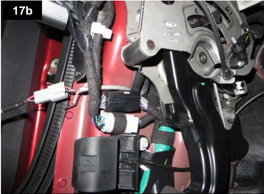
KEEP WIRE CLEAR OF E-BRAKE. ONCE WIRE THROUGH FIREWALL.
