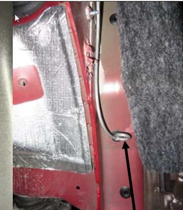
After rubber grommet installed on harness-"O" or "O1",
