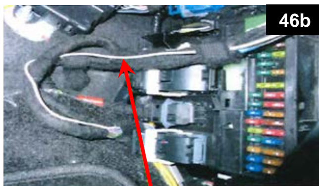
Run-start secured to BCM J1 harness
