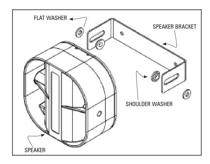
For 200 Series Sirens the speaker must be electrically isolated from the vehicle's chassis ground.
