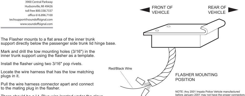
There should be a Lt. Blue wire located under the glove compartment. This is the flasher on/off wire. Connect the Lt. Blue wire to a switch. Connect the other end of the switch to a source of +12Vdc.
