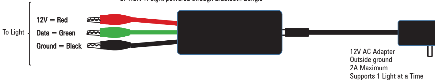
OPTION 1: Light powered through Bluetooth Dongle
